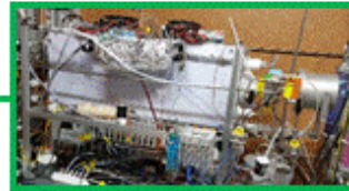
KNU flow reactor Controlled aging (1-5 d)
